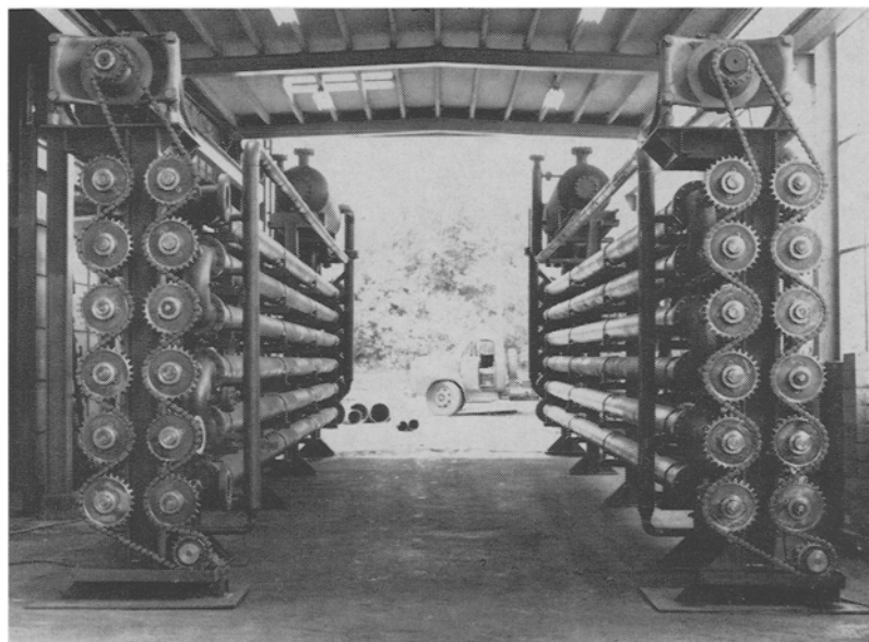
2 Stands of 12 Shells Each, 6" Inner Pipe, All Steel, Drive Cabinet Removed. De-waxing Lube Oils.
